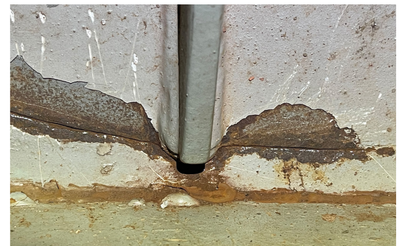
Opposite page: Liebherr cranes at port This Page: Top: A crack was observed at the connection between the portal beam and the leg. Middle: A crack near a structural connection. Bottom: Richard Phillips, mechanical engineer at CPA
